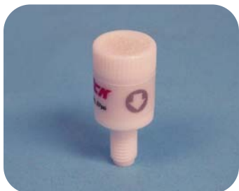
DV-115 Air Inlet Evaporation Control Valve, PTFE with Viton seal, 0.07 psi cracking pressure
