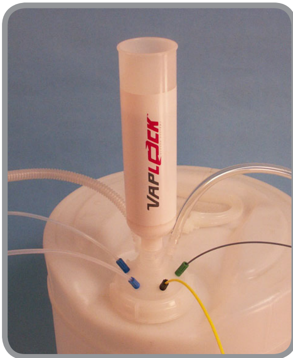
SV-165 and SV-165NAL 70mm (Hedwin) and 70mm (Nalgene) 7-ported manifolds with free-spinning cap collar; with (5) 1/4-28 ports, (1) 1/2" NPT port
