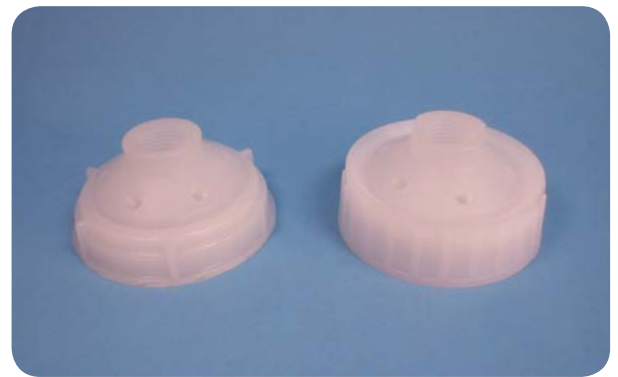
SV-165 and SV-165NAL 70mm (Hedwin) and 70mm (Nalgene) 7-ported manifolds with free-spinning cap collar; with (5) 1/4-28 ports, (1) 1/2" NPT port
