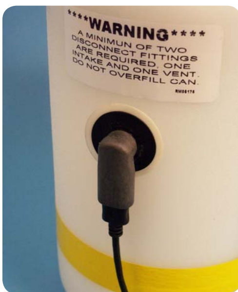
LS-102 Sensor head connected to Polyethylene tank
