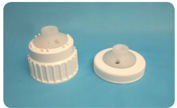
SV-215 and SV-225 83B Nalgene (left, SV-215) and 100-415 Nalgene (right, SV-225), with free-spinning cap collar and 10 ports: (1) 1/2" NPT, (3) 1/4" NPT, and (6) 1/4-28
